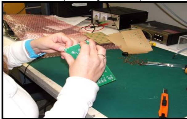
Checking a board mounted switch
